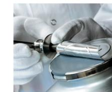
Stainless steel cap opener allows to smoothly open the aluminium cap without touching it, thus avoiding the risk of contamination or cutting the glove.
