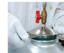
Connected with reduced vacuum source, the stainless steel removal/insertion tool allows to insert/remove the chlorobutyl plug easily (no rubbing nor effort) and avoids any contact with the plug (reduces risk of contamination).
