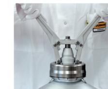
2nd generation stainless steel crimping tool provides reinforced crimping efficiency and still higher reliability of sealing. It is easy to sterilise and does not require maintenance nor adjustment. An automation of this manual tool can be studied upon request.
