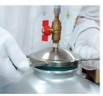
Connected with reduced vacuum source, the stainless steel removal/insertion tool allows to insert/remove the chlorobutyl plug easily (no rubbing nor effort) and avoids any contact with the plug (reduces risk of contamination).
