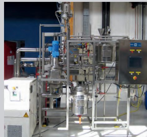
30L subcritical extractor - 22 bar pressure
