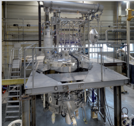
Direct steam distillation of dry powder under pressure.
